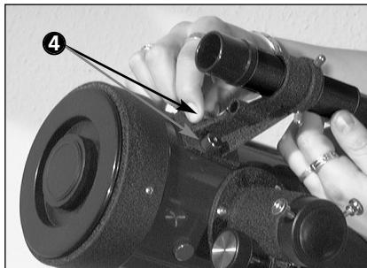
To mount the finder scope (2) you must first loosen the fastening screws (4) for the finder. Hold the finder scope with the objective in the same direction as the telescope, place onto mounting and retighten the screws carefully.
