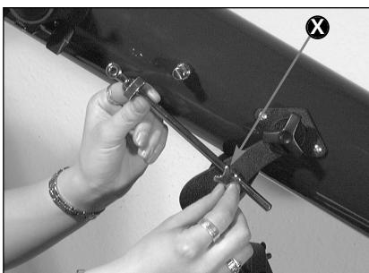
To install the vertical fine adjustment (2), first you put the adjusting pole through the mounting of the vertical fine adjustment (X) on the mount.
