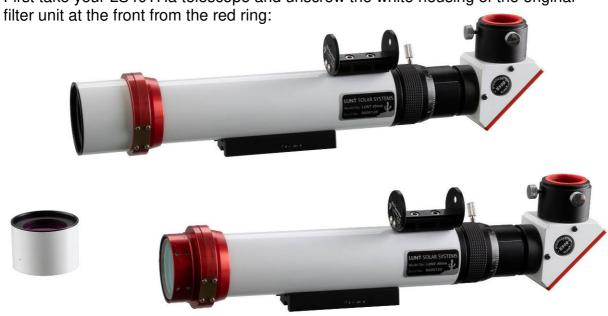
Now take the LS40FHa double-stack filter and also unscrew the white housing from the red ring:
