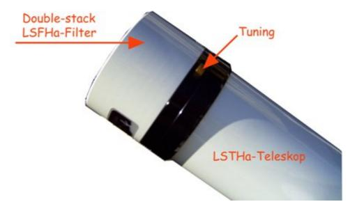
It can happen that you will see the following picture in your eyepiece, after you have your double-stack filter screwed on. Then you just have to tune your double-stack filter to move the sun reflexes out of your field of view.
