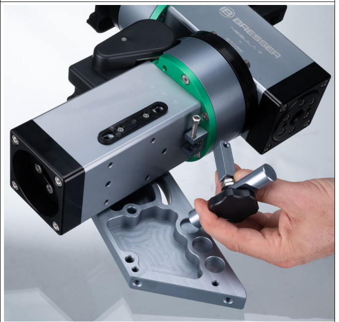
Put back the mount base flange previously removed and fix it tightening carefully the four M8 bolts.
